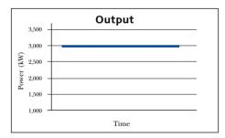
V90-3.0 MW allows the rotor speed to vary within a range of approximately 60 percent in relation to nominal rpm. Thus the rotor speed can vary by as much as 30 percent above and below synchronous speed. This minimizes both unwanted fluctuations in the output to the grid supply and the loads on the vital parts of the construction.
